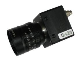
The image sensor has a Multi-Slope Exposure mode that prevents over-exposure of brighter parts of an image while preserving contrast in the darker areas. In this way the dynamic range is extended from the normal 60dB up to 90dB. The camera can be switched between normal and Multi-Slope mode.
